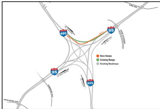
ABOVE: NEW SOUTHBOUND I-95 TO WESTBOUND I-695 RAMP
